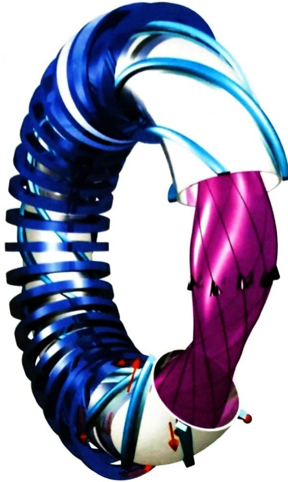
Magnetic field only by external coils
